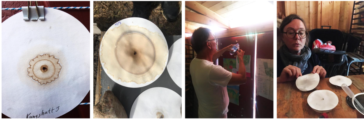
Figure 2: Left: Fully developed soil chromatograms. Right: The process of conducting soil chromatography.
