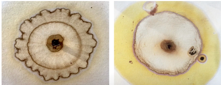
Figure 1: Left: a chromatogram of fertile soil. Right: a chromatogram of infertile soil.
